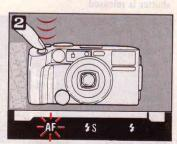
② Press the shutter release button fully to start the self-timer.
